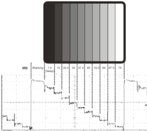
The purpose of the color temperature setup is to assure uniform gray level from black to the brightest scenes. If a uniform gray screen is displayed, no matter the brightness level, no tinting in either red, green or blue direction should be apparent. This is known as “color tracking”. Once the proper color temperature is set, AKB will maintain the cutoff of the CRT to assure proper low light performance.
