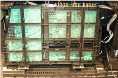
6. To place chassis tray back into the cabinet, align the bottom of the chassis tray with the locking mechanism of the bottom cabinet assembly.
