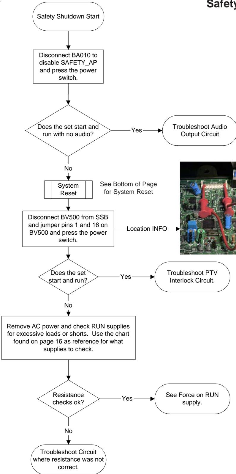
**System Reset:** Remove AC power and short out CP555 for 10 seconds then reapply AC power. See page 11 for details.
