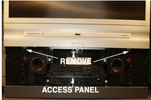
4. Access Panel may now be removed to allow service of Kine Drive circuits.
