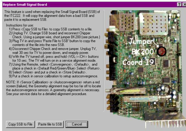
3. Follow the instructions on this screen to copy the alignment data from the defective SSB to the new SSB.
